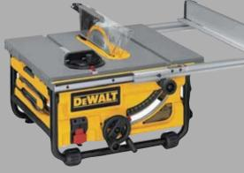
10" Jobsite Table Saw 15 amp. Rack & Pinion fence design delivers consistent fence- to-blade parallelism. Metal roll cage base and 16" of rip easily cuts a variety of larger shelving and trim materials. 3,850 RPM, 10" blade diameter, 5/8" arbor, 2-1/2" dust port diameter, 3-1/8" depth of cut at 90 degrees, 2-1/4" at 45 degrees. Model DW745
