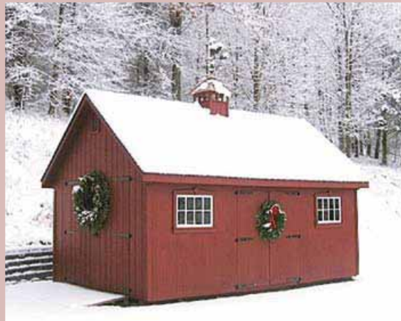
12' x 20' Board and Batten with 10 Pitch Roof
