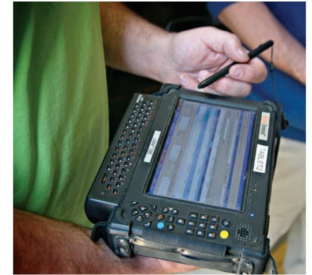
in barcode reader—runs on Windows and operates the same bisTrack software as all the other computers within the company. It even shows the standard screens that the counter salesmen see. The device is made to handle the wear and tear of life in the lumberyard, as well as do its job even in cold New England winter mornings.
