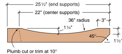
**End seat supports** Trim four 2x4s to 25½ inches. Attach the inside seat supports to the rear and front legs so they rest on the top edge of the 2x4 main braces. Attach the outside seat supports level with the inside ones.
