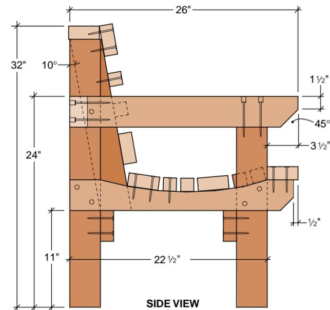
**4. Seat supports** The curved seat supports are made up of 2x4 lumber sandwiching either the 4x4 rear legs or the single 2x4 backrest support. To shape the curve, make a template for a 36-inch radius cut. Mark the cut to start 3 inches in from the front. Use a bandsaw to cut the radius to a depth of no more than 1¼ inches. Finish the seat supports with a 45° bevel cut to match the armrests.
