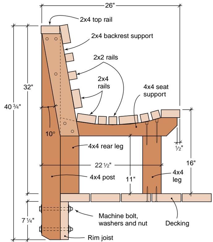
**3. Backrest supports** Trim both ends of each 2x4 double backrest support to 10°. Attach flush to the top of each 4x4 post and to the 4x4 seat supports.
